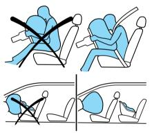
All occupants of the vehicle including the driver should always properly wear their safety belts even when air bag SRS is provided.
